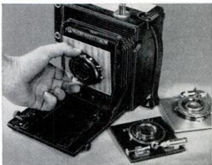
Below, left, without disturbing the locked positions, use the range finder in the normal manner and note the footage scale. Then rack out the lens and set this footage on the scale for the lens of longer focal length as below
